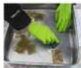
samplers get fouled and need to be cleaned
