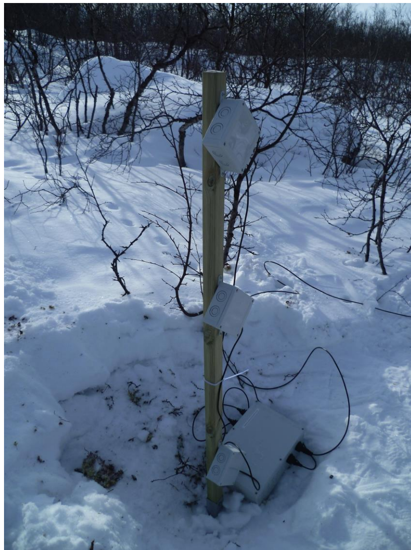
Figure: One of the poles with three sensors attached and the testbed box.
