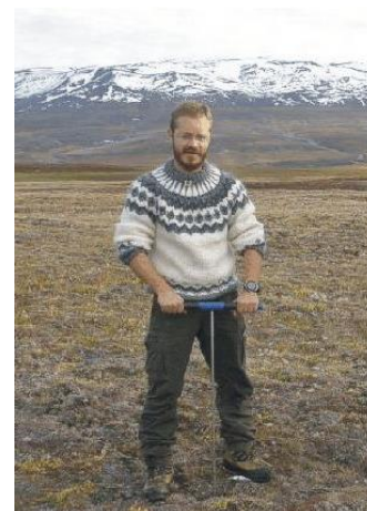
Active layer measurement using probe (Hanne H Christiansen/UNIS)
