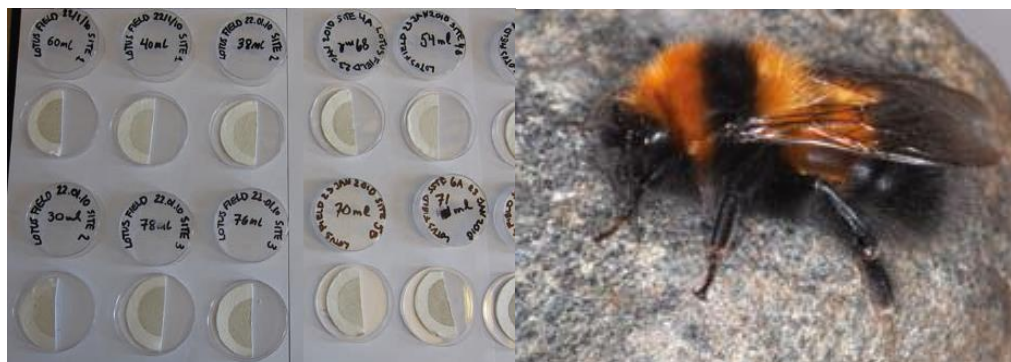
Figure 7. Transnational projects that aid environmental protection and conservation: left, filters from a thermo/optical carbon aerosol analyser (cut in half) showing dark half circles where tiny black carbon particles from snow melt water have darkened the filter (C.A. Pedersen et al. in INTERACT Stories of Arctic Science); right, the bumblebee Bombus hyperboreus , one of the vulnerable species studied at Toolik Lake, Alaska, to understand bumblebee diversity and abundance (B. Martinet et al. in INTERACT Stories of Arctic Science).
