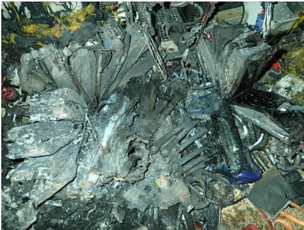
Figure 26. Burned out lithium batteries on a workbench where nearby batteries have been ignited from the others.
