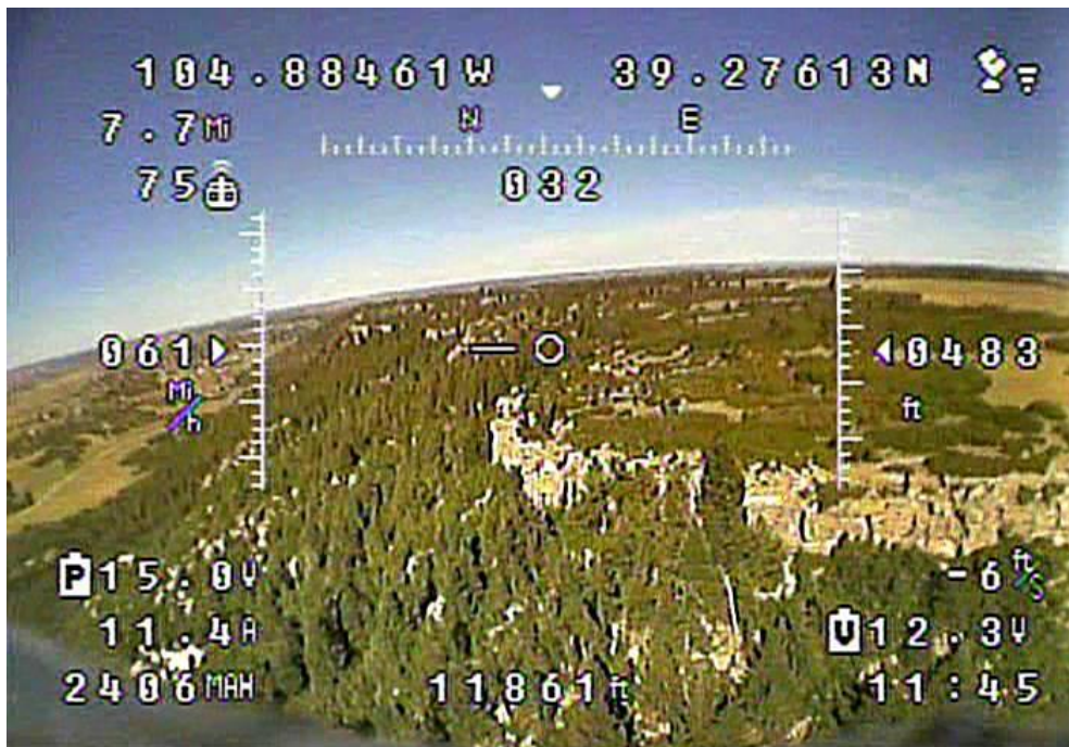
Figure 28. Typical FPV video feed with on-screen display (OSD). Creative Commons, Patrick McKay.
