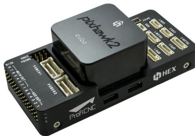
Figure 18. A Pixhawk 2 flight controller from ProficNC.
