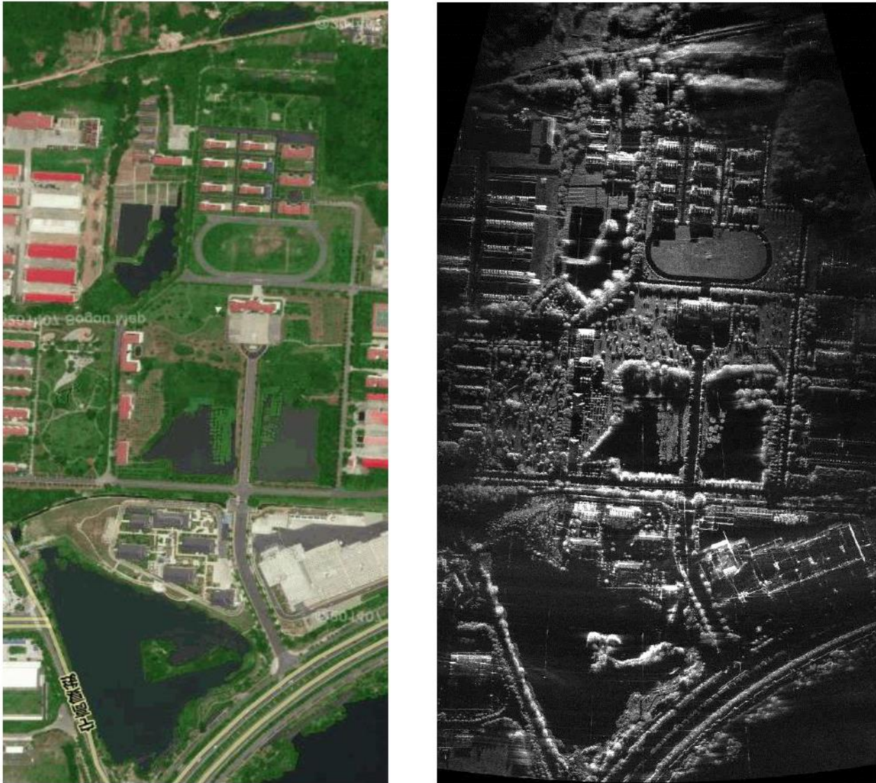
Figure 66. Comparison of an optical image (left) and a SAR image constructed from a drone system (right).
