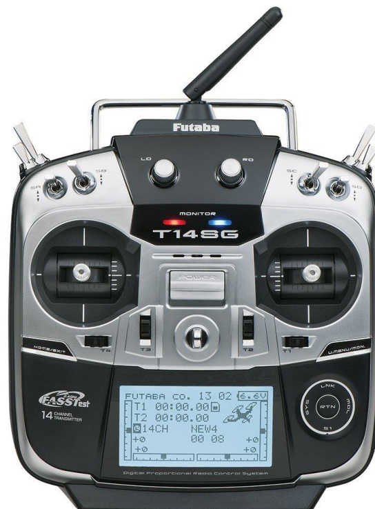
Figure 20. An advanced remote controller from Futaba.
