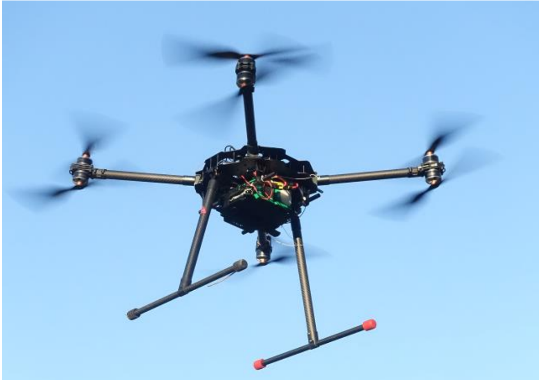
Figure 13. An octocopter configured as X8 with two rotors on each arm.
