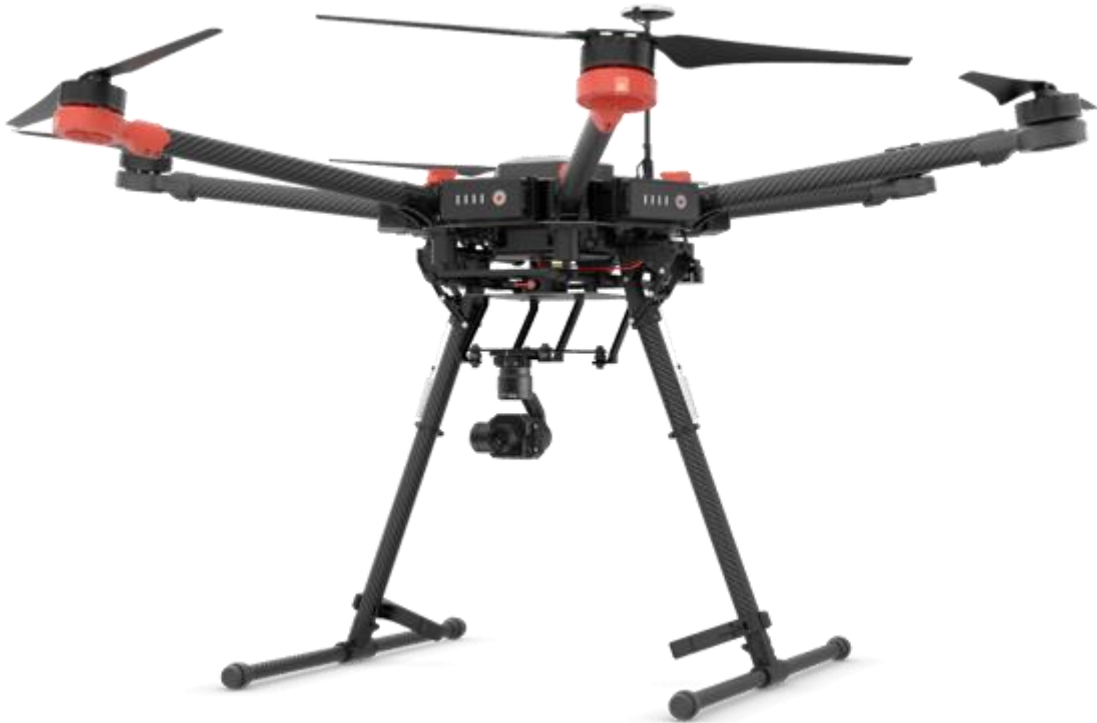
Figure 59. M600 from drone manufacturer DJI and the integrated IR-camera from FLIR (DJI, 2017).
