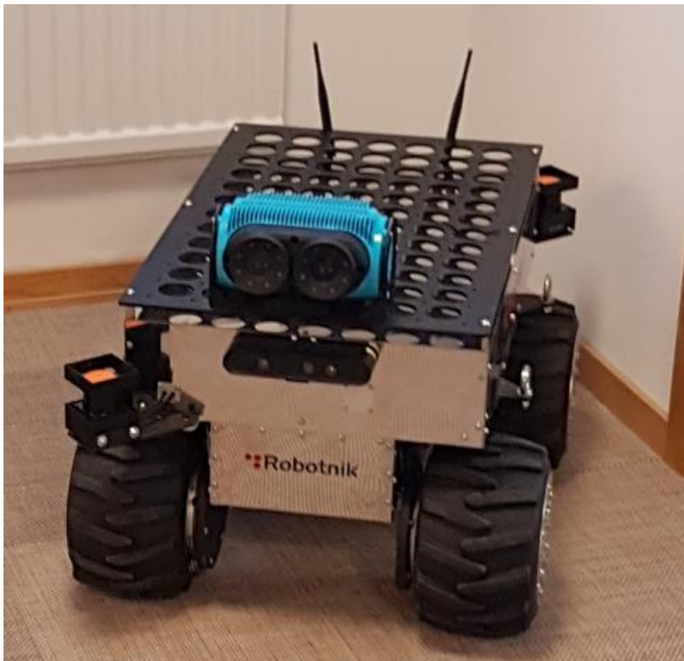
Figure 2. Intelligent Vision System (Unibap, 2017) on a wheeled robot (Robotdalen, 2017) developed to be used in the agriculture area to identify and mechanically remove unwanted weeds from the wanted crops.
