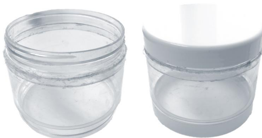
Figure 7. A picture demonstrating the designed laboratory bottle threaded in both ends.
