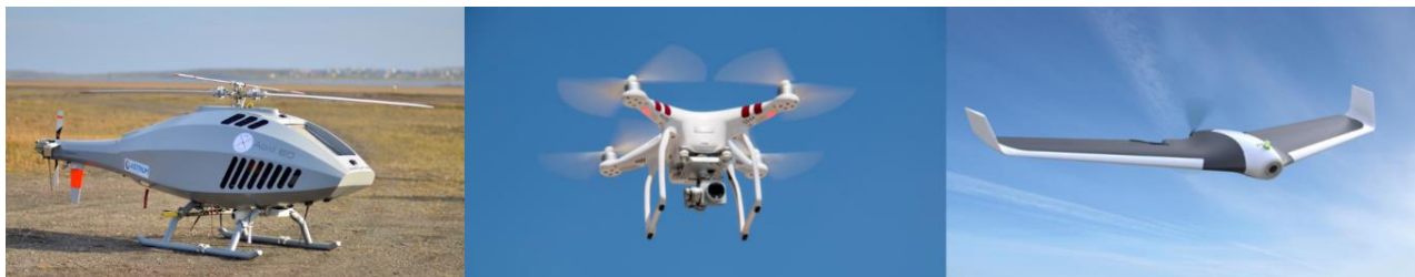
Figure 1. Three different types of drones. From left: rotor helicopter, multirotor, and fixed-wing.
